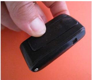
To fit it in properly use your thumb and apply combined rubbing and pressing movements to press the web into the grooves.
