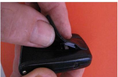
Once first button sits in properly in the cut out, you will repeat the same fitting process for the second cut out.
