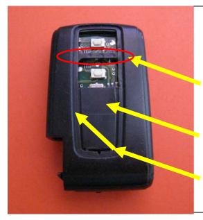
With flat screwdriver lift sides of the soft rubber pad and remove it from the shell. Do not insert screwdriver inside the shell as you may damage electronic switches.
