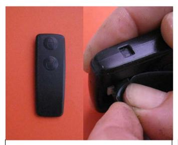
Start fitting pad from the **top** (**lock button cut out**) by slightly bending and sliding it under the sides of the cut out.
